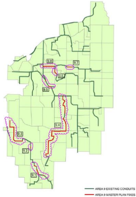
(b) Area of existing / future sewer deficiencies (Analysis performed in 2007)
