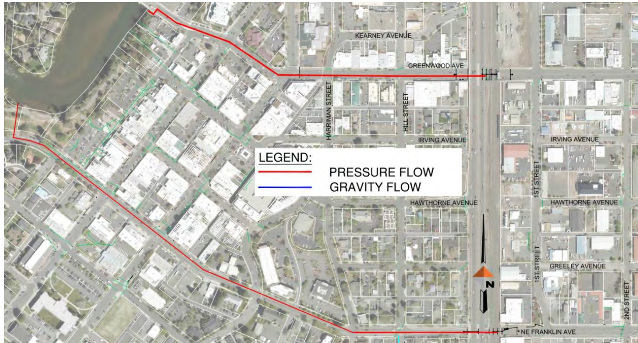
Figure 28. Individual outfalls to the Deschutes River.
