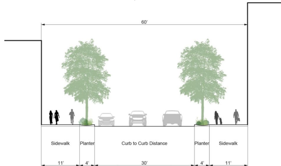
Figure 61. Draft Local Street Cross-Section Concept
